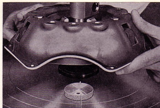
Fig. 16. Placing the clutch in the fixture, I 1. Packing blocks No. 0
